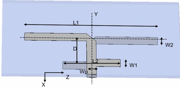
Fig. 2. DPDA Layout and Geometrical parameters
