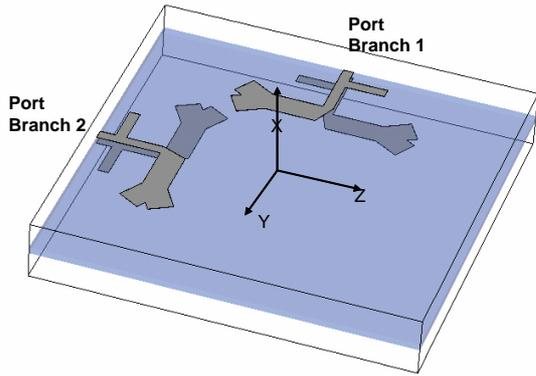
Fig. 8. Polarization diversity antenna using two PF-DPDA's
