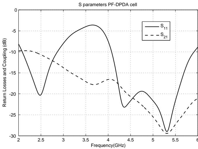
Fig. 9. Coupling between cell elements in polarization diversity schema
