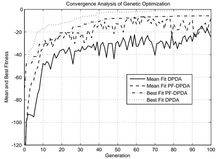
Fig. 3. Genetic Algorithm Optimization features for the antenna problem
