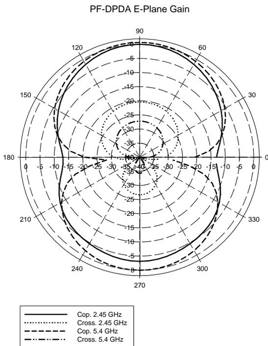
Fig. 5. Gain Pattern of PF-DPDA Antenna
