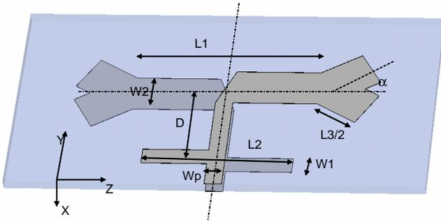
Fig. 1. PF-DPDA Layout and Geometrical parameters
