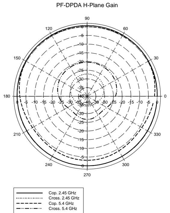
Fig. 6. Gain Pattern of PF-DPDA Antenna
