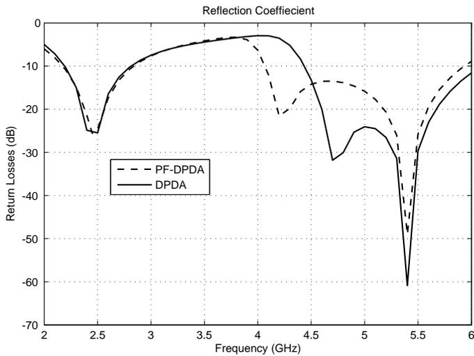
Fig. 4. Return Losses of DPDA and PF-DPDA
