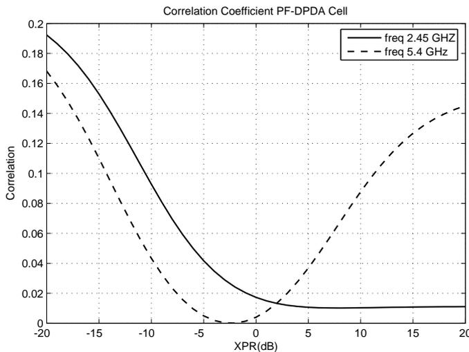
Fig. 10. Correlation between cell element antennas
